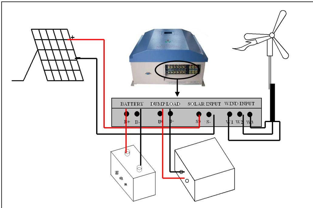
After wind/solar hybrid generator system and the various components of photovoltaic panels installed and the construction of the external circuit completed, the following order should be carried out to make the connection and operation safely and reliably.
