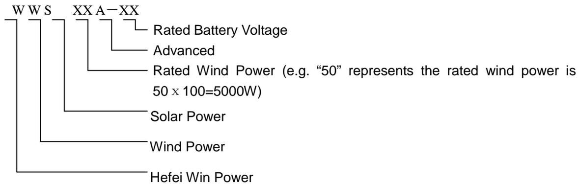
eg. WWS 50A-48 (5000W Advanced Wind/Solar Hybrid Controller, Battery Voltage is 48V)
